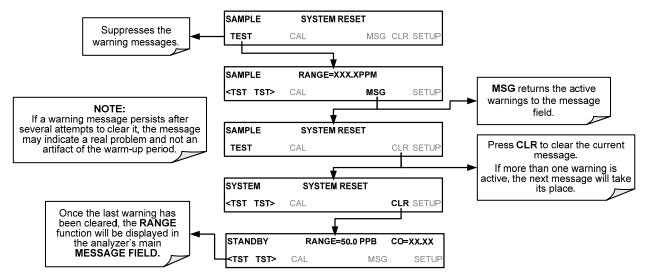
Figure 4-3: Viewing and Clearing GFC7001T/GFC7001TM WARNING Messages
